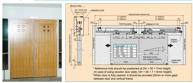
Avoid strong impact cause of damage with any parts. Operate door in upper position than half of door height. Not available door pocket use.
